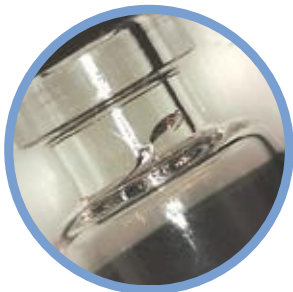
Crimp & neck defects
